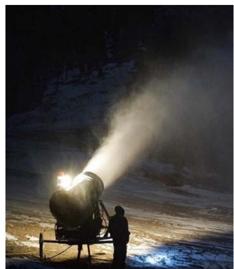
Water is atomized at a very high pressure to make snow that allows the resort to open.
