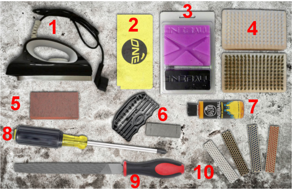
Properly maintain your equipment regularly. Tools needed for waxing include (1) Iron, (2) Scraper, (3) Snowboard or ski wax, (4) Nylon and Brass Brush, (5) Gummy Stone, (6) File Guide, (7) Base Cleaner, (8) Phillips Screwdriver, (9) File, (10) Diamond Stones.
