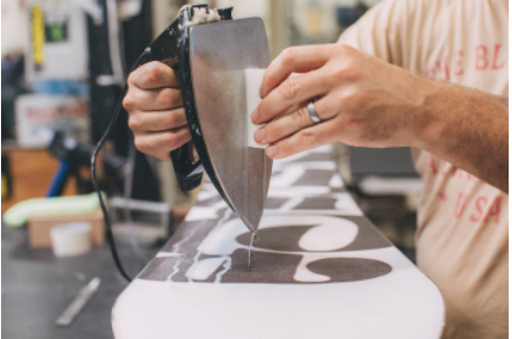
Technician uses hot iron to melt the wax that is applied to your skis or snowboard.
